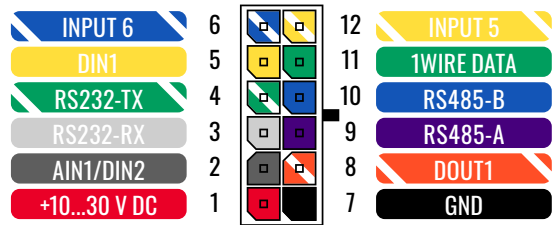
FMC225 2x6 socket pinout
