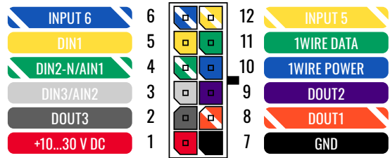
FMC130 2x6 socket pinout
