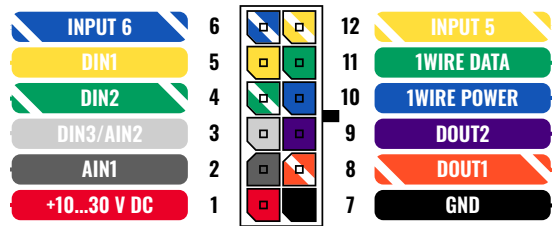
FMB122 2x6 socket pinout
